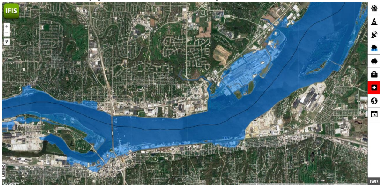
Flood inundation maps for Lock and Dam No. 15 upstream of Davenport at a scenario-based flood stage of 26 feet.
